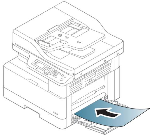
3. Squeeze the multi-purpose tray paper width guides and adjust them to the width of the paper. Do not force them too much, or the paper will bent resulting in a paper jam or skew.
