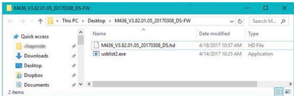
3. Drag the firmware file M436\_V3.82.01.05\_20170308.hd and drop it on top of the usblast2.exe file. This will start the firmware download to the printer.
