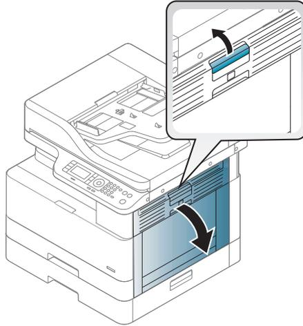
2. Remove the jammed paper from the transfer roller assembly.
