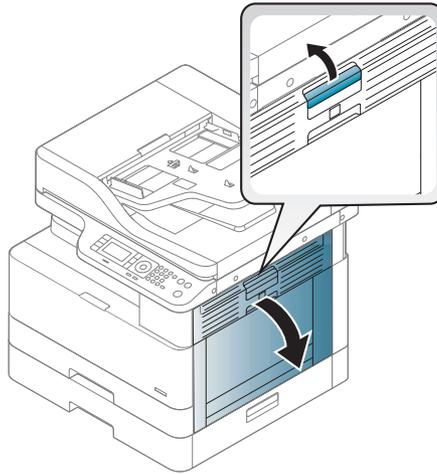
2. Open the jam guide and remove the jammed paper.
