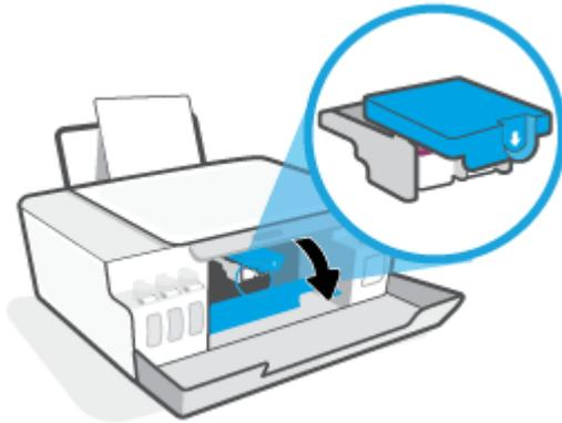
5. Push down to open the printhead latch.
