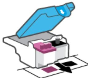
7. Clean the printhead contacts and printer contacts.
