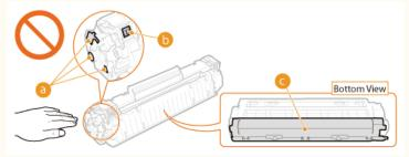
The toner cartridge is a magnetic product. Keep it away from floppy disks, disk drives, and other devices that can be affected by magnetism. Failure to do so may result in data loss.
